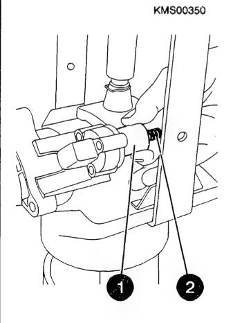
STARTING MOTOR ASSEMBLY Assembling solenoid switch Slip on solenoid switch and attach to drive-end bearing. Pav attention to mark. Use torque wrench. Torque wrench: comm. avail.
